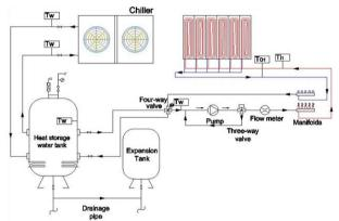
**Figure 7.** Hydraulic circuit of the test system
