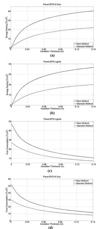
**Figure 10.** Total energy saving versus insulation thickness for SDDM and NDDM a) Natural Gas b) Lignite, fuel consumption comparison of the methods c) Natural Gas d) Lignite
