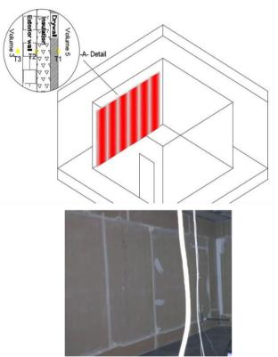
Figure 6. Arrangement of the wall mounted radiant panel
