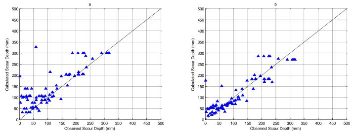
Fig. 6: Scatter diagrams for observed and calculated scour depths a) Breusers equation b) Improved Breusers equation.
