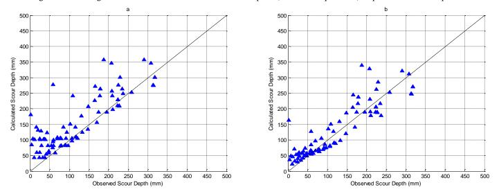
Fig. 7: Scatter diagrams for observed and calculated scour depths a) Jain equation b) Improved Jain equation.
