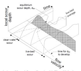
Fig. 3: Variation of Local Scour Depth with Flow Velocity and Time [3].
