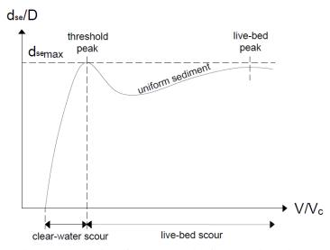
Fig. 2: The variation of scour type with flow velocity ratio [5].
