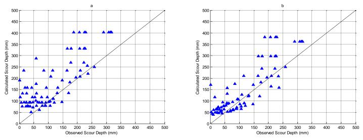
Fig. 5: Scatter diagrams for observed and calculated scour depths a) Laursen equation b) Improved Laursen equation.
