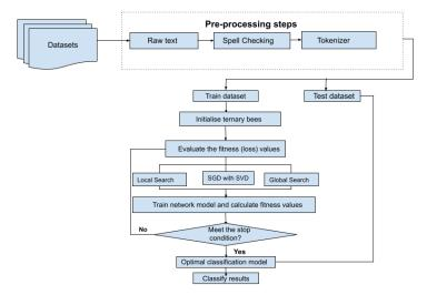
Figure 4. Flowchart of the proposed classification model.
