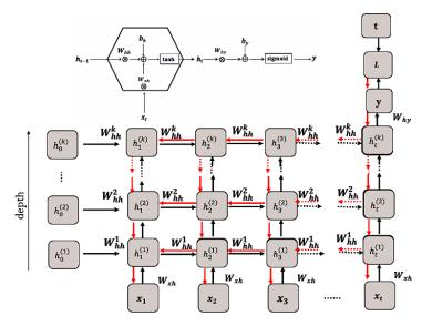
**Figure 1.** A Deep RNN architecture representing a bee in the proposed algorithm. Black lines are the forward pass of RNN cell at time t (unfolded version at upper) and red lines representing the error backpropagation through long-term dependencies.
