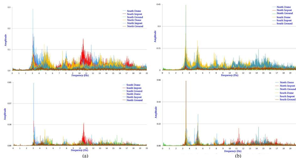
Figure 4. Fourier (above) and Power (below) Spectrums, a) Perpendicular to Qibla-x b) Qibla-y direction, (OMA-1).
