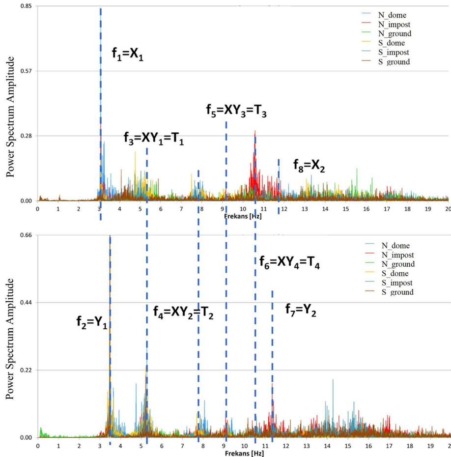
**Figure 5.** Comparison and matching of the spectrums for  $x$  and  $y$  directions (OMA-1).
