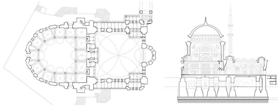
**Figure 2.** Ground floor plan and section through courtyard-mihrab direction of the mosque.
