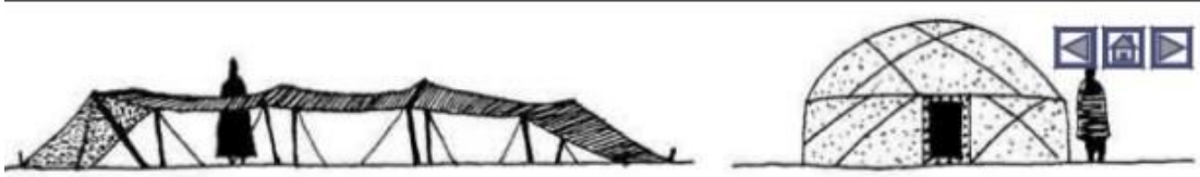
FIG. 2.5. Portable tents of sticks and felt. Left: Arab tent. Right: Mongol Yurt.
