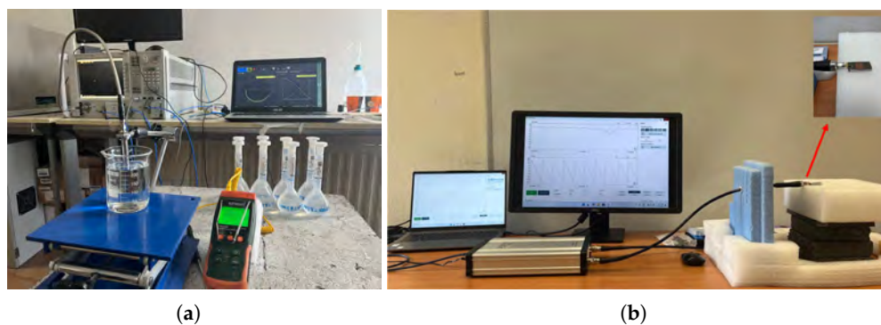
Figure 3. Photos of experimental setup for (a) complex permittivity and (b) |S_{11}| measurement.
