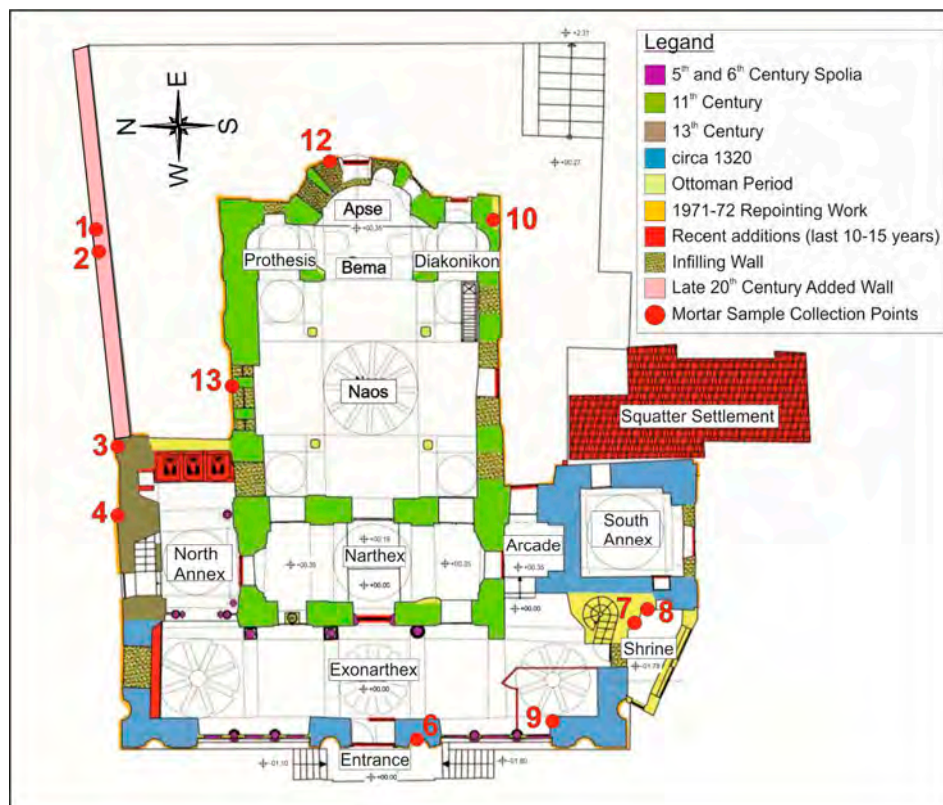
Figure 2. Architectural plan of Vefa Kilise Mosque and the chronological representation of its structural elements (modified from [20]). The analyzed laying mortars are marked with red dots, and sample numbers are indicated.
