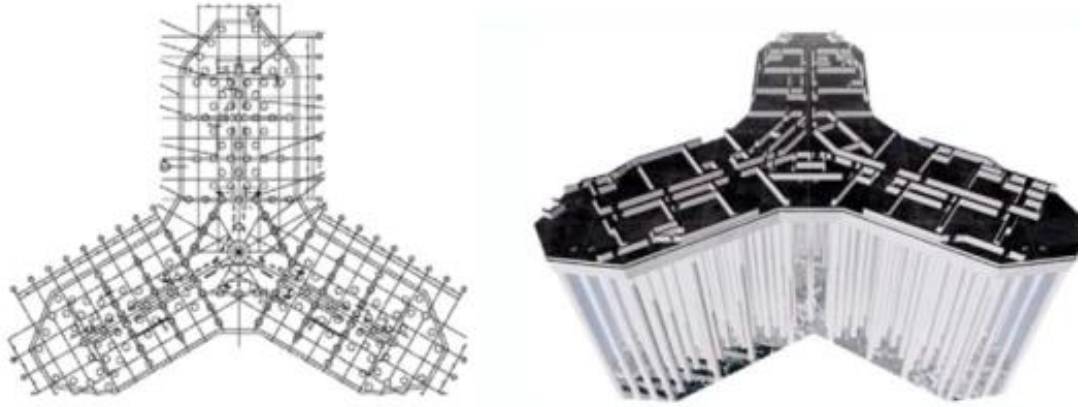
Resim 4.12: Burj Khalifa temel sistemi (Abdelrazaq, 2011; Smith, 2020)
