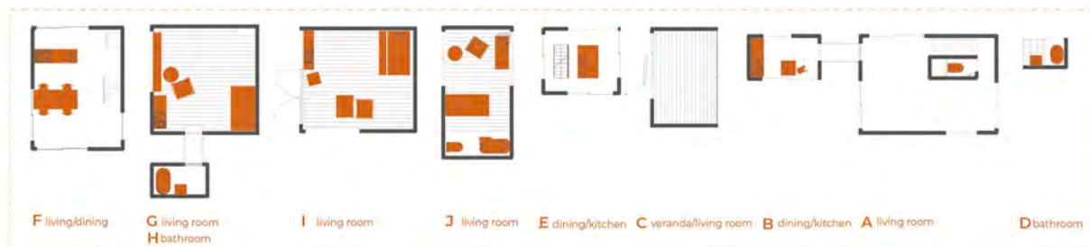
Fig. 6 The adaptable interior furnishings of different units in Moriyama House.
