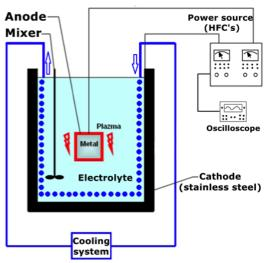
Figure 1. The schematic diagram of the MAO device.
