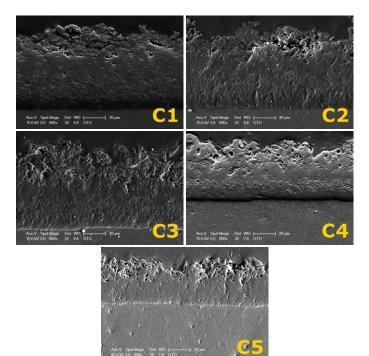
Figure 7. A cross-sectional morphology of the ceramic coatings.
