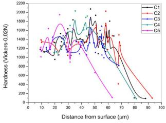
Figure 5. Vickers hardness profiles of the coatings fabricated under different anode-cathode pulse duration couples.
