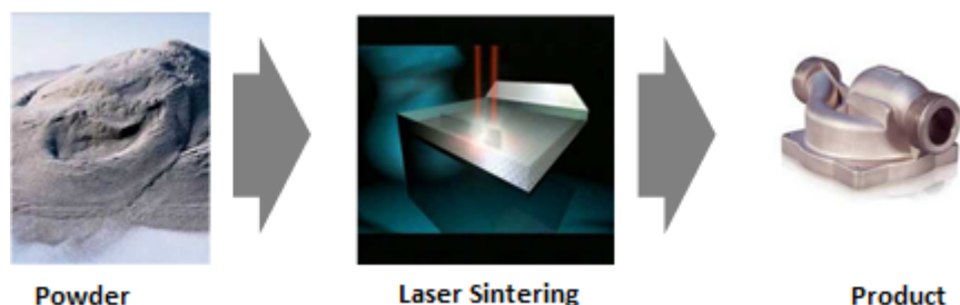
Figure 1 Direct metal laser sintering (DMLS) production method from powder to product [1].
