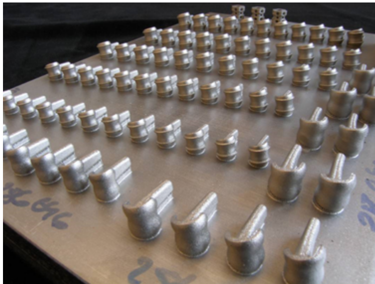
Figure 7 Batch of finger implants in EOS CobaltChrome MP1[2].
