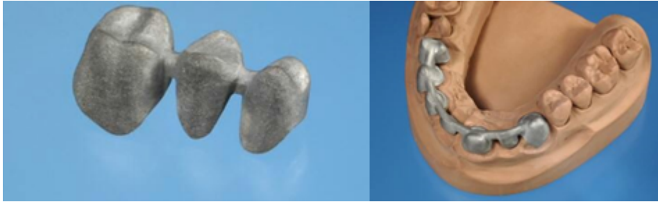
Figure 6 Direct Metal Laser Sintering (DMLS) CoCrMo alloy for dental applications [2].
