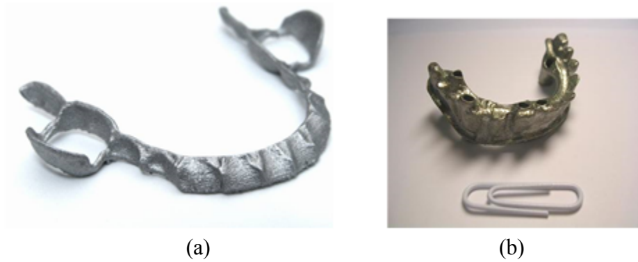
Figure 11 Dental applications. (a) Aligner in EOS CoCr MP1, (b) Dental device in EOS Titanium Ti64 [2].
